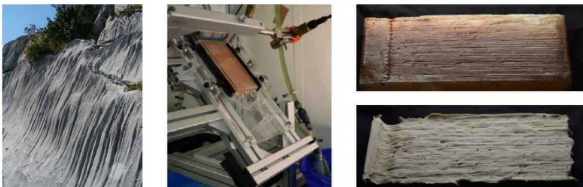
Figure 1: Reproduction in the laboratory of the longitudinal pattern created by thin runoff flows on a soluble inclined
